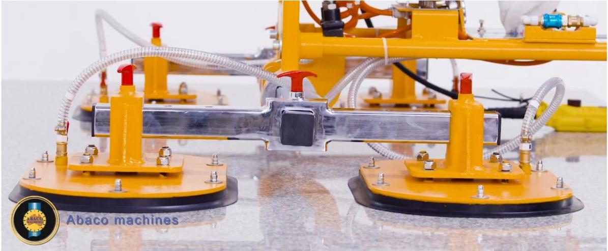
7. By design, there is a gap between the suction base and the base plate. Do not tighten the nuts on the suction base to seal this gap. A large spring is housed inside the suction base to relieve the weight of the entire SVL device as it is placed on a surface. The gap serves as a buffer for the spring to engage.
